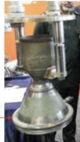
Simorgh steering engine combustor without nozzle extension ?
